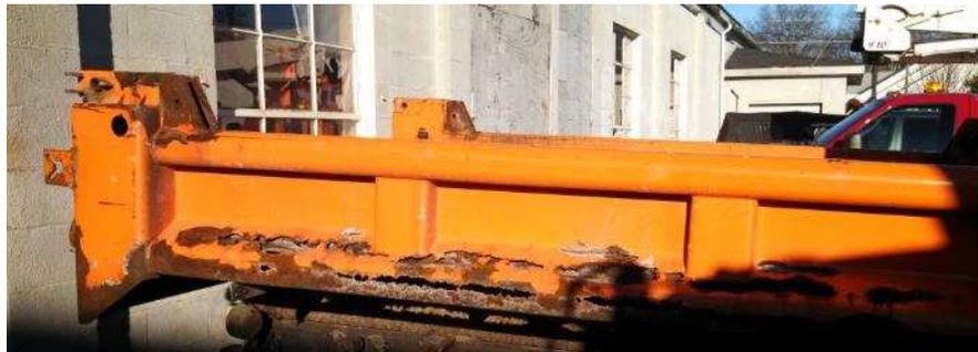
Outdoor storage contributes to accelerated equipment deterioration
