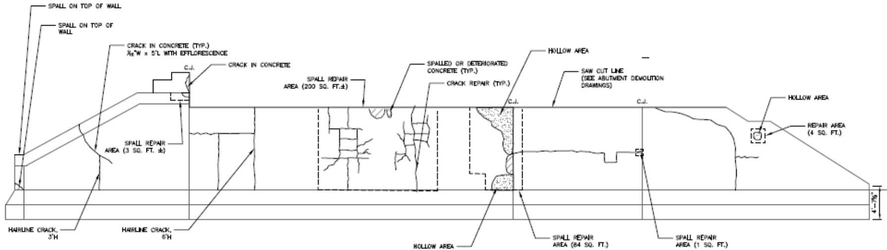
Cracks, Spalls & Hollow Areas Throughout
